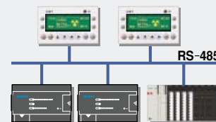
XGT Panels can control different devices of which protocol is equal.
